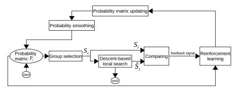
Figure: A schematic diagram of PLS for grouping problems. From a starting solution generated according to the probability matrix, the process iteratively runs until its stopping condition is met Jin-Kao Hao Learning-driven optimization
